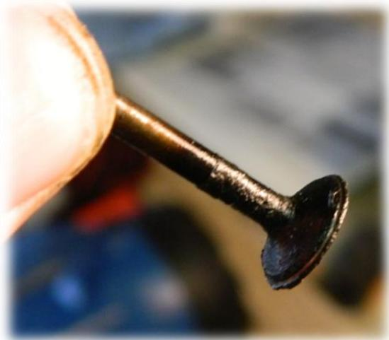
Well, this looked to be the problem. I got the old dremal metal brush and cleaned her up. I also cleaned up the head where the valve seats. In my excitement I forgot to take a picture of the cleaned valve. Trust me, it is a world of difference.
