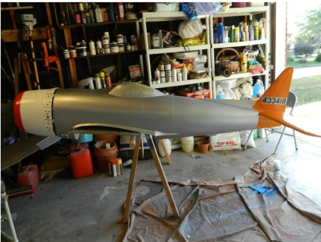
I always mount my fuse and wing in a saw horse rotating jig. Makes painting much easier.
