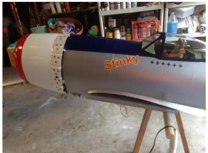
First view of wheels on the ground. I always love this part, you know you are getting close when you have wheels on the ground. All electronics and retracts passed functional. Next I'll mount the engine and tank.
