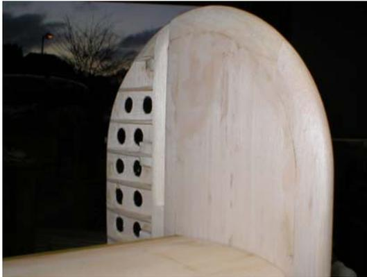
Next I will final sand all the structures and glass with .5 oz/yd cloth. I use West Epoxy at full strength for the first coat and west diluted 50% with alcohol for the second flow coat. Herman found out the West Epoxy recommends using acetone instead of alcohol because the the quicker flash time for acetone – Hummm, makes sense.
