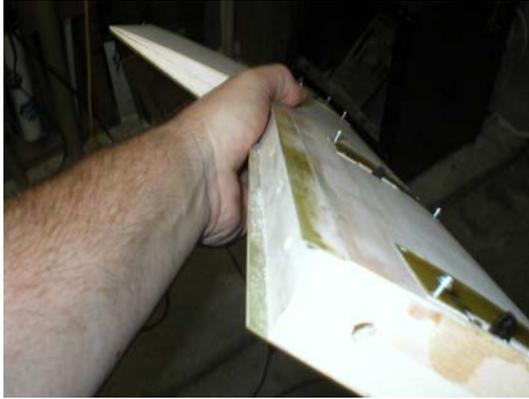
Last but not least, the tail structure assembled, showing the lightning holes on the rudder.
