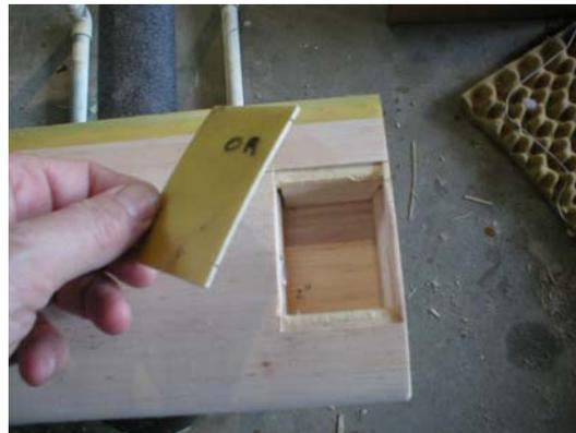
This photo shows the hatch in its proper place. The tail has four servos and four hatches, one each left, right, elevator and rudder.
