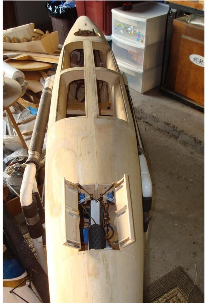
The servo mechanism for the gear door.
