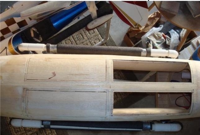
All four doors open and the gear door mechanism functional.
