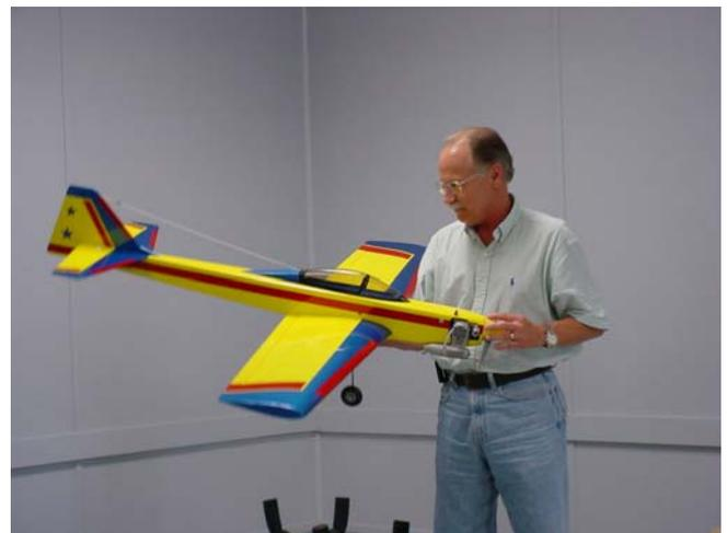
James Lemon brought in a plane to show that was under construction. It is a T2A Mark IV with a fiberglass fuse and foam wing.
