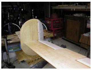
Finally, the tail empennage ready for priming.
