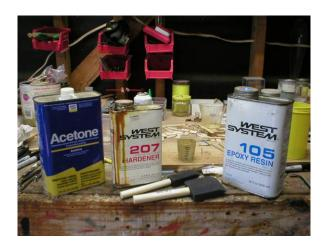
The first layer of West epoxy will attach the cloth, the second, thinned 50% with acetone (some thin the first coat also) fills the weave. The set of pics show the first weave, brushing on the second coat, and the final results in the curing stage.
