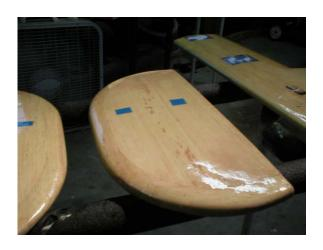
For the tail feathers I used Solartex from Balsa USA. This is a cloth covering that stretches as good as or better than traditional covering. The picture below shows the cloth ready to be ironed on.
