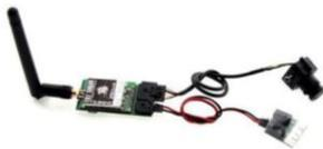
Left is the total hardware package for the transmission side of the FPV. It has the camera, the transmitter, the antenna, and the power board altogether. The best part is you can take it out of one plane, heli, copter and put it in another one very easily.
